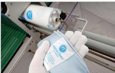
World leading Teknek Nanoclean™ cleaning core. Nanoclean™ is a silicone and static free system that is capable of cleaning particles smaller than 1 micron. Ideal for thin, sensitive materials such as polyimide, polyester, copper etc.
